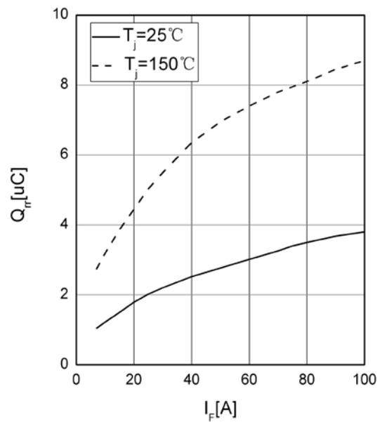
**recovered charge of Diode, Inverter (typical)**
