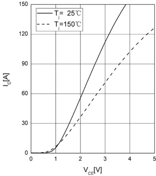
**output characteristic IGBT, Inverter (typical)**
