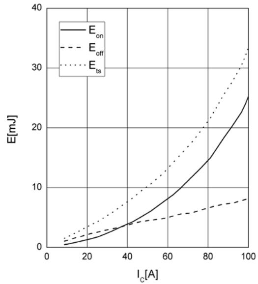
**switching losses IGBT, Inverter (typical)**
